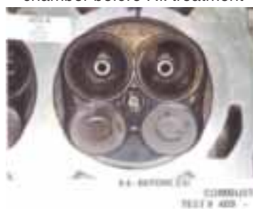
Picture F - Combustion chamber before P.i. treatment
