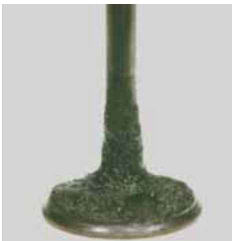
Picture D - Intake valve before P.i. treatment
