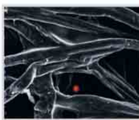
Cellulose fibers are inconsistent in size and shape: more contaminants pass through: restriction is higher and holding capacity is lower.
